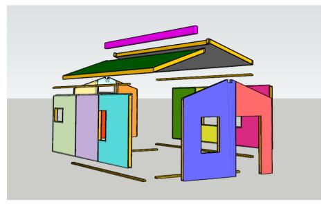
Shell package: Wall: 4.5" (114mm) SIPs, R-value 16; Roof: 6.5" (165mm) SIPs, R-value 24, glulam beam and other accessories necessary for shell.
