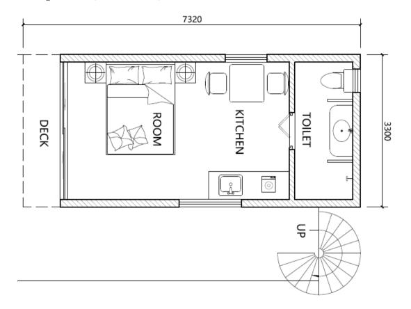
Wall: 6.5" (165mm) SIPs, R-value 22; Roof: 8.25" (210mm) SIPs, R-value 29.
