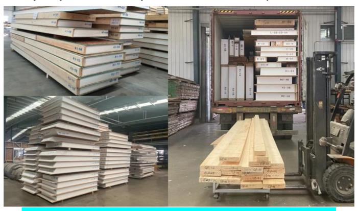
1x 40'HQ container can load components of a SIPs house in around 100 m2.
